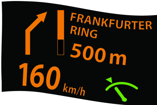
HUD image showing distortion for improper installation or adjustment
